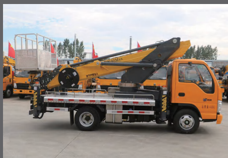
Basket static hydraulic automatic leveling, 360° rotation, overload automatic protection.
