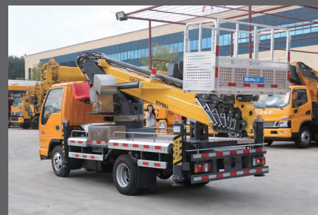
The outrigger is equipped with position detection switch and automatic induction alarm function.
